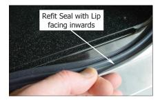
f. Press the door seal into the locating groove in the front face of the oven until the seal is properly located all around the oven.
